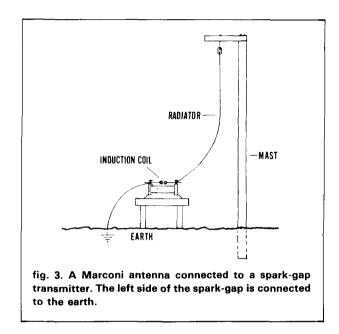
tion and returned home to begin work on what was to become the wireless telegraph, or what we now call radio. Marconi soon began experimenting with antenna placement and eventually came to connect one side of the spark-gap in his transmitter to a vertical antenna (see **fig. 3**) and the other side of the gap to the earth or ground.
